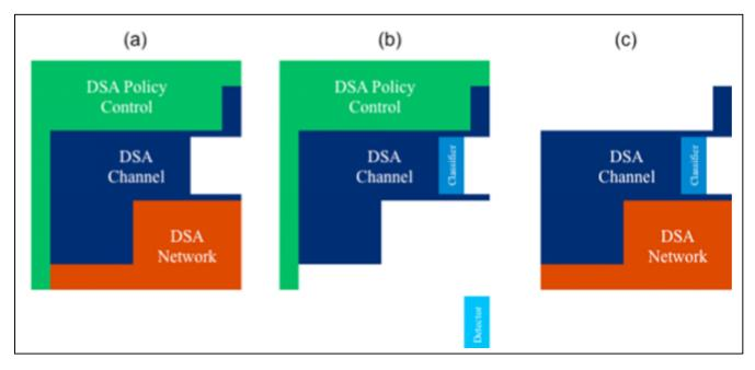
Fig. 3. (a) DSA implementation without detector and classifier; (b) DSA implementation with sepearte detector and no network module; (c) DSA implementation without policy control and without detector.
