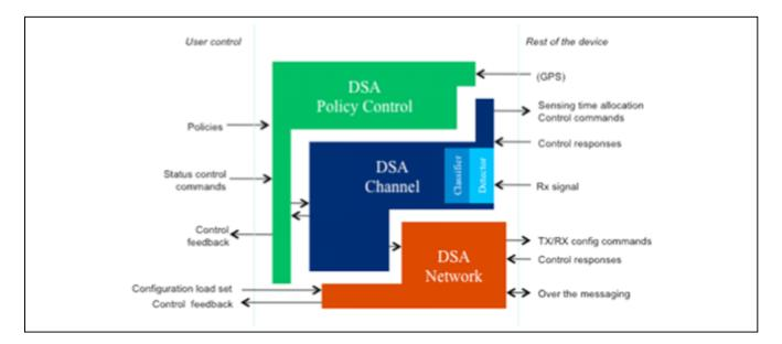
Fig. 2. Complete fully-integrated DSA implementation consists of a policy control module, channel module with detector and classifier, and network modules.
