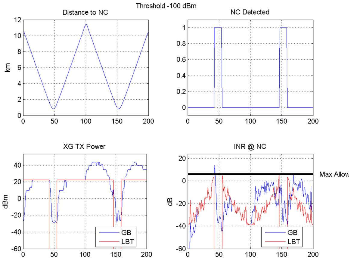
Figure 12. Group Behavior algorithm vs. LBT, measured over the same test course and time-aligned.
