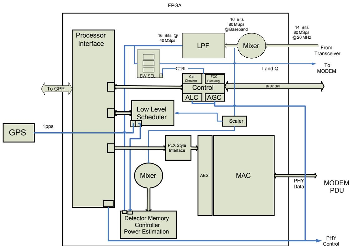
Figure 8. FPGA Architecture Contains Multiple Functions
