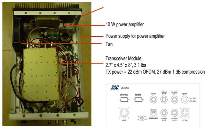
Figure 9. Complete DSA Radio w/Power Amplifier
