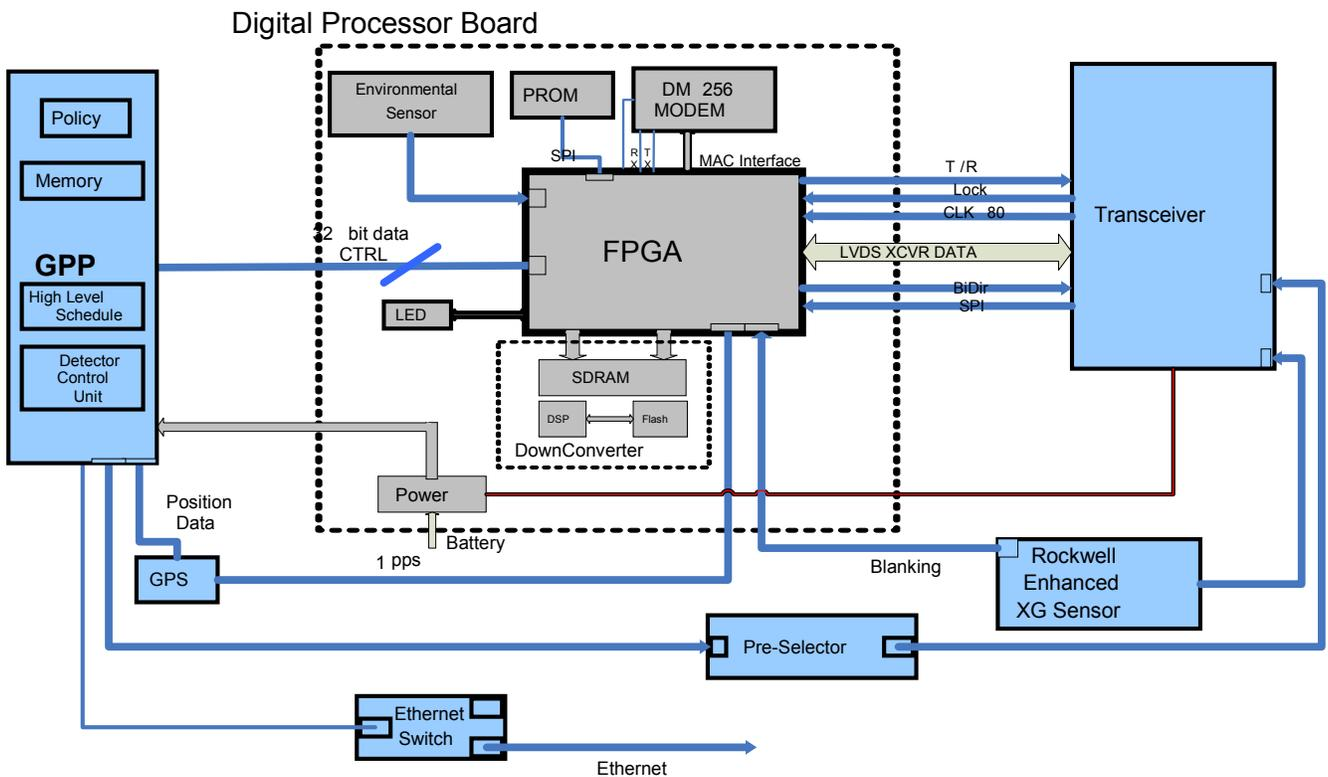
Figure 7. Digital Processing Board Architecture
