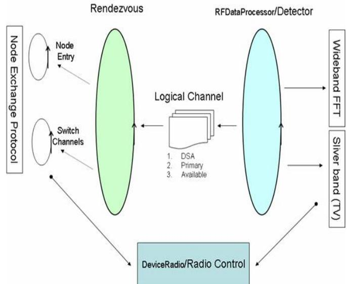
Figure 2. High-Level DSA Process Flow
