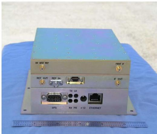
Figure 6. RF Transceiver Module (DSA 1000)
