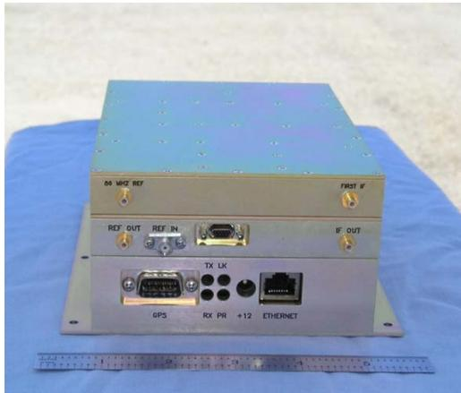
Figure 6. RF Transceiver Module (DSA 1000)
