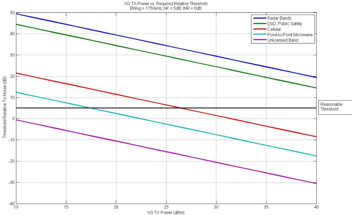
Figure 10. Required detector performance versus DSA transmit power level for different use cases.
