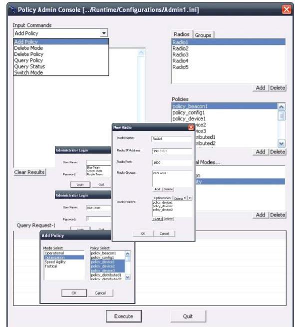
Fig. 9. A snapshot of the administration tool used to disseminate policies onto XG-enabled radios.
