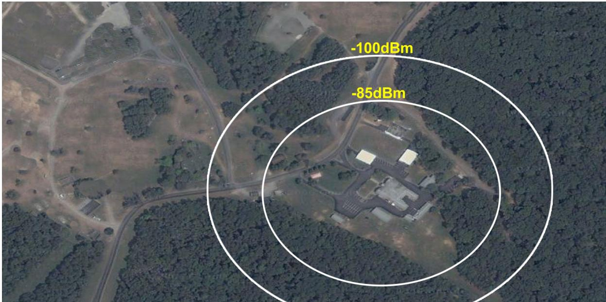
Fig. 7. In Scenario 3, policy dictates different detection thresholds for different channels, with implications for detection range as shown here. In the actual demonstration, thresholds were adjusted in advance to make the best use of the test range available (so -85 and -100 dBm are just given as examples).
