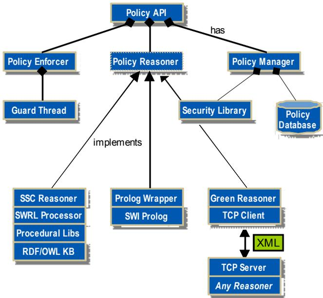
Fig. 2. XG Policy Conformance Components interact with the XG System Strategy Reasoner via Policy API, which allows for the development of additional PCCs either integrated within the XG software or as an external application communicating through an XML-based protocol.
