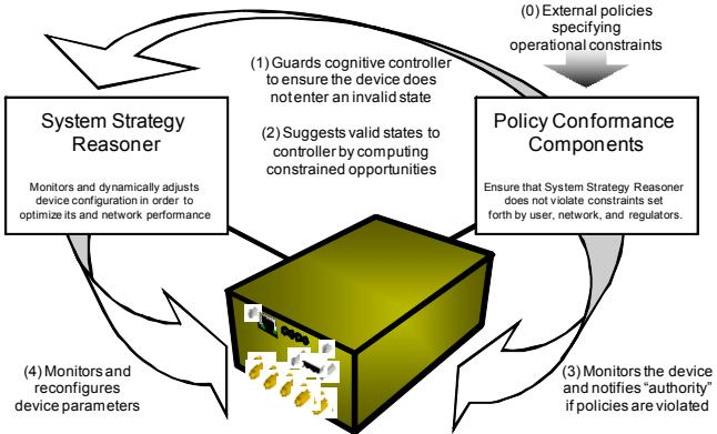
Fig. 1. XG-enabled cognitive frequency-agile device includes a cognitive System Strategy Reasoner for monitoring and adjusting the device for balancing its performance and Policy Conformance Components for providing operational spectrum access assurance to stakeholders.
