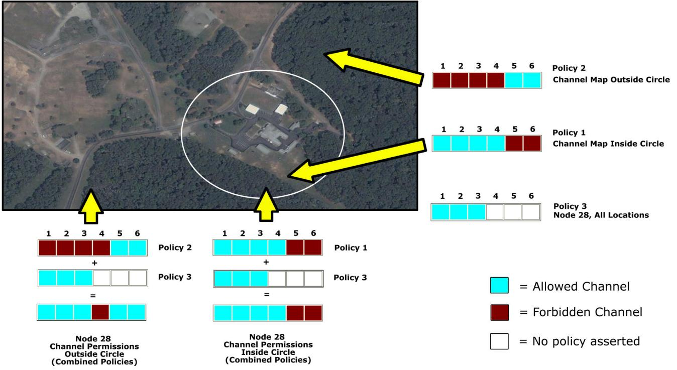
Fig. 8. In Scenario 4, policies dictate usage of different channels based on radio's current location. Within the circle, radios are permitted to use only channels 1 through 4 whereas outside of the circle radios are permitted to consider channels 5 and 6. Additionally, for this scenario we have re-introduced a third policy, which enables a radio to use channels 1 through 3 anywhere, anytime provided the radio does not interfere with other signals possibly present on those channels.
