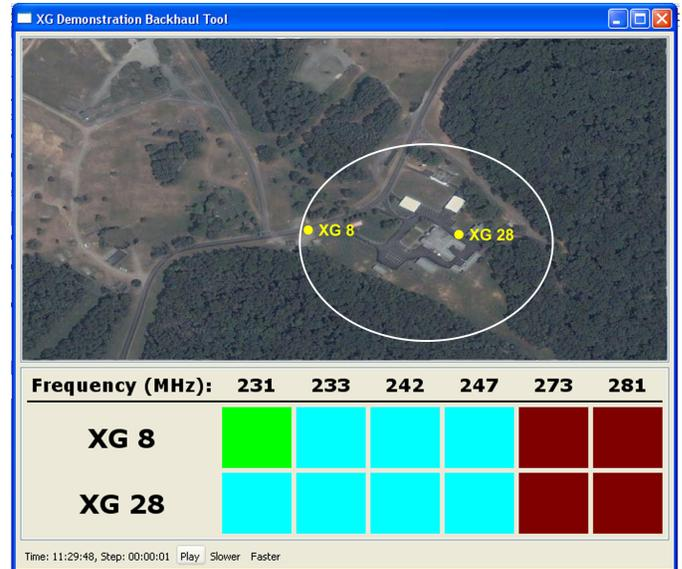
Fig. 6. A screen snapshot of the demonstration backhaul tool showing the current position and spectral map of a pair of XG-enabled devices. Permitted, unused channels are shown in teal; active channels in bright green; and prohibited channels in brick red. The perimeter used for the location-based policy demonstration is seen here in white.
