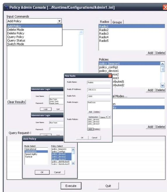
Fig. 9. A snapshot of the administration tool used to disseminate policies onto XG-enabled radios.
