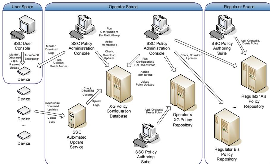
Fig. 3. For enabling each and all spectrum stakeholders to define and manage their spectrum access requirements, the system includes authoring and controlling tools used to manually and automatically assign spectrum access rights in terms of policies to XG-enabled cognitive frequency-agile radios.
