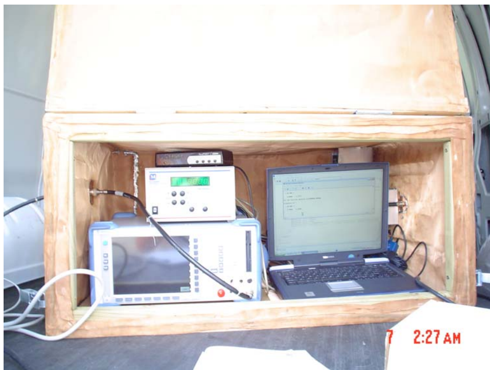
Figure 2: RF Shielded Enclosure Used With the Spectrum Analyzer and Laptop Computer
