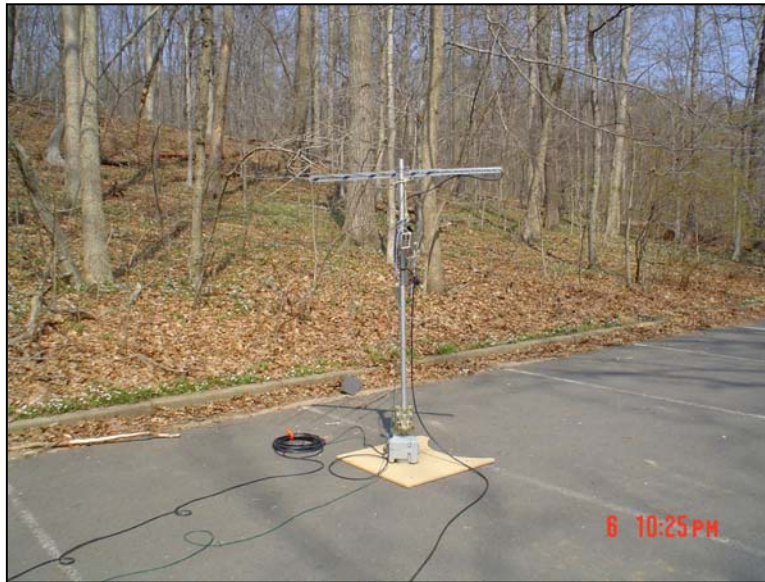
Figure 5: Directional LPA Antenna (used for frequencies below 1,000 MHz)
