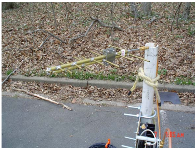
Figure 7: Small LPA Antenna and Pre-Amplifier Used for Frequencies Above 1 GHz
