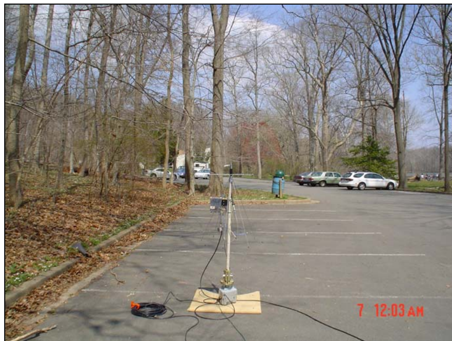
Figure 4: Omni-Directional Discone Antenna (used for frequencies below 1,000 MHz)
