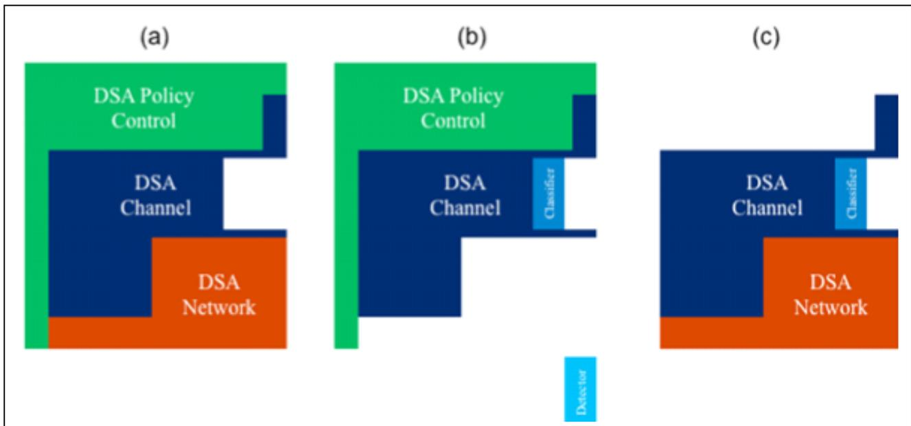
Fig. 3. (a) DSA implementation without detector and classifier; (b) DSA implementation with sepearte detector and no network module; (c) DSAimplementation without policy control and without detector.
