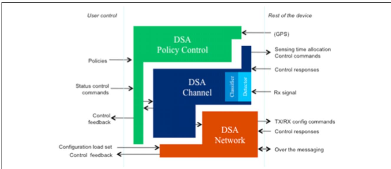
Fig. 2. Complete fully-integrated DSA implementation consists of a policy control module, channel module with detector and classifier, and network modules.
