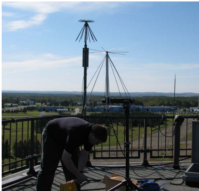
Figure 3. Discone Antennas Used to Take Measurements
